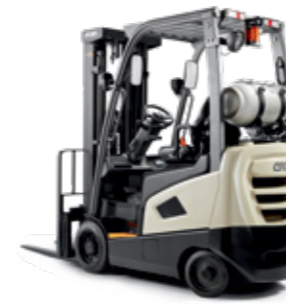
C-G Series, Models 15-20 Tire: Cushion Power: Internal Combustion - LPG Load Capacity: 1500 to 2000 kg Lift Height: 1980 to 6000 mm
