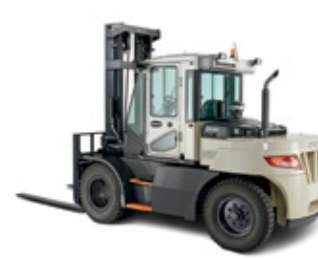
C-D Series, Models 60-90 Tire: Pneumatic Power: Internal Combustion - Diesel Load Capacity: 6000 to 9000 kg Lift Height: 3000 to 6050 mm
