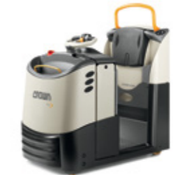
TC 3000 Series Tow Tractor Load Capacity: 3000 kg
